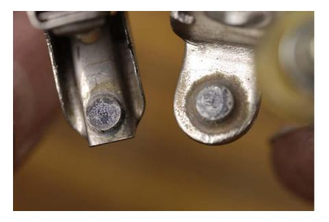
There is the case that dirt such as oil deposited on the points makes them rough, but in fact, it is often caused by a broken condenser. These points need to be replaced, but...
