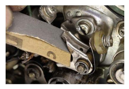
Let's open the points in the position where the points heel is not on the cam lobe and look at the points. If the points are burned or rough, fold sandpaper in two, and sandwich it, and brush back and forth the contact point. Use #600 sandpaper.
