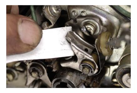
If oil sticks to the points, the contact surface may burn, causing the electricity not to be conducted. This may cause idling malfunctions and acceleration failure. Spread the points with your fingertips and sandwich a paper and pull it out.
