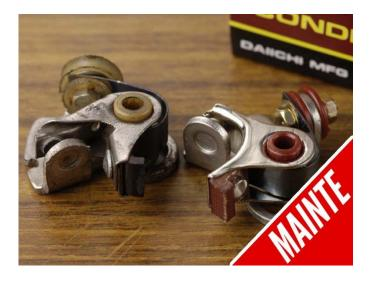
The most important thing is understanding the ignition circuit. But... the contact breaker (points) ignition system is often used in vintage models, and often referred to as the cause of malfunctioning. In the case of the contact breaker (points) ignition system, if you understand the ignition circuit, you can recover quickly even if you get into trouble. At the same time, it's helpful to keep in mind what happens when the points and condenser are out of order.
