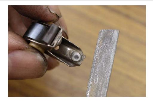
It is better to replace the points with a new one, if it's too rough. But if you want to fix it as an emergency measure, polish the contact point. The points are opened, and use sandpaper (#320) folded in two, and sandwich it and polished the contact point.
