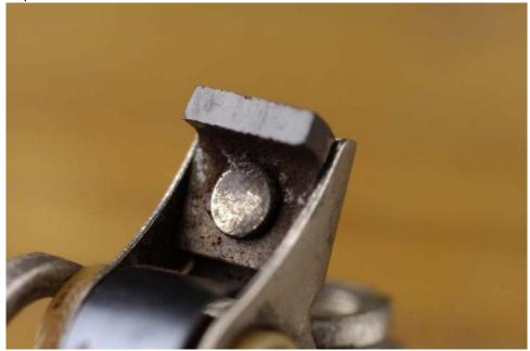
In some cases, the points heel is made of bakelite is reduced, so the proper point gap may not be obtained. To prevent the reduction of the heel, lubricated it with points grease.
